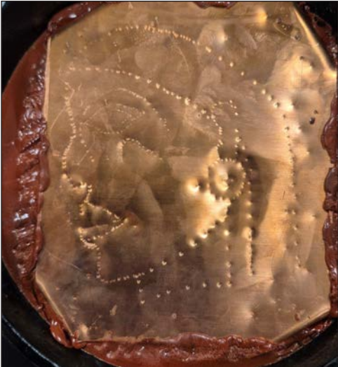
The copper sheet is put into the jeweler's pitch, and an outline of the design is made by tapping dots.
