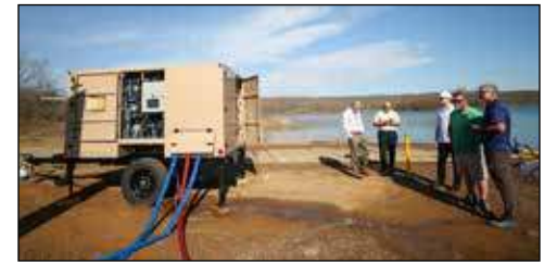
The ROWPU can convert 508 gallons of water to drinkable water per hour.
