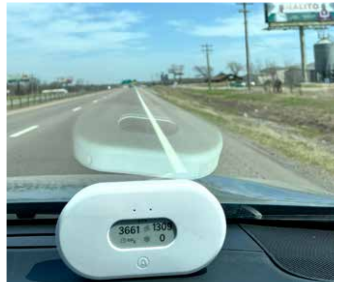
Photo by Kendra Germany-Wall After a 30 minute drive from Sherman to Durant the CO2 levels in the car were over 3000 parts per million (ppm). According to www.CO2meter.com levels between 2,000 and 5,000 ppm can cause headaches, fatigue, stuffiness, poor concentration, loss of focus, increased heart rate and nausea.
