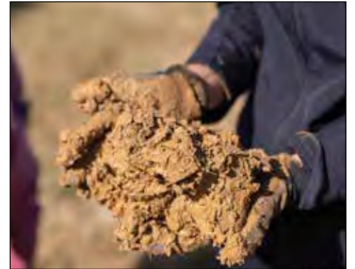
A mixture of dirt, straw and water is used to create the clay thrown against the side of the traditional shelter and spread by hand for insulation.
